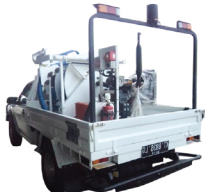
Pump Crew Unit
